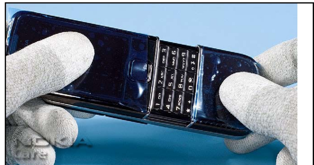
6. Shift open the assembly.
